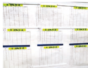
Task management charts for each machine show how much has been cut for each product, and based on this instructs how much should be cut for the next production batch.
